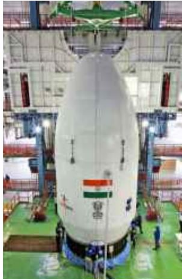
Ready to fly: The ISRO on Wednesday integrated the Chandrayaan-3 spacecraft with Launch Vehicle Mark-III at the Satish Dhawan Space Centre in Sriharikota. SPECIAL ARRANGEMENT
